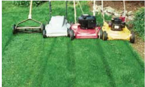
You can grasscycle with any mower. Push mowers (left) and conventional power mowers (right) leave clippings on the surface to break down. Electric and gas mulching mowers (center) blow chopped clippings down to the soil, leaving a clean lawn.
